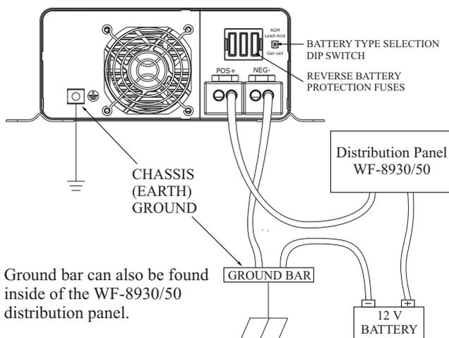
Ground bar can also be found inside of the WF-8930/50 distribution panel.
