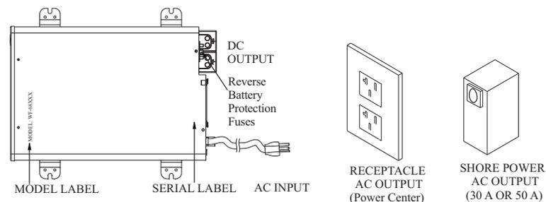
If the reverse polarity fuses are blown, it means the RV battery was accidentally connected in reverse, either at the battery or at the converter. Reconnect properly, then replace the fuse with the same type and amp rating as the original ATC automotive-style fuse.
